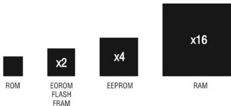
Fig. 2. Comparative sizes of memory boards of different types with a size of 1 bit per chip
