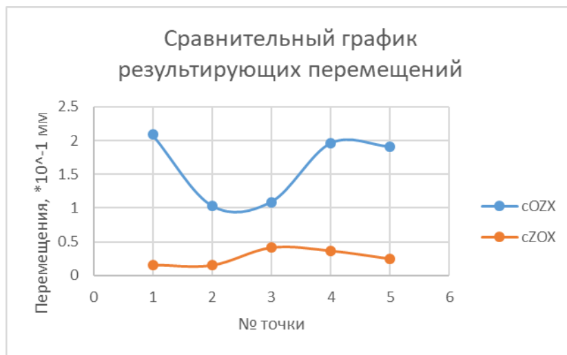
Figure 10 - Graphs of the resulting displacements of the layouts with OZX and with ZOX
